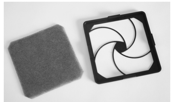
Figure 5-1. The back cover snaps off for access to the foam filter. The filter can generally be rinsed out, dried, and replaced if it is only clogged with dust.
