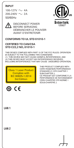
Figure 3-1. CDRH and IEC 60825-1:2014 regulation compliance label. See Power Cords and Disconnecting Power on page 13 for more information about disconnecting power before servicing.
