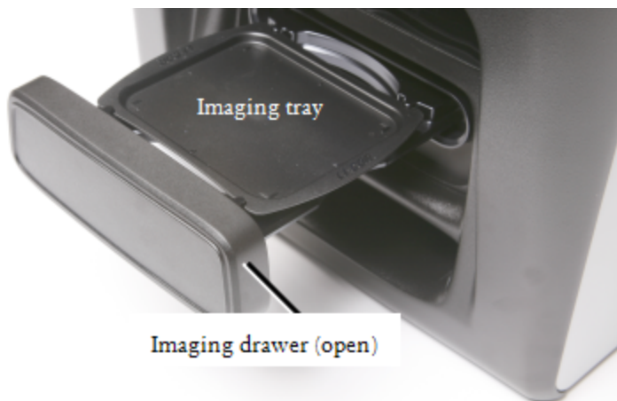
Figure 4-5. The imaging drawer holds one imaging tray that is capable of containing one membrane or gel up to 10 x 12 cm.
