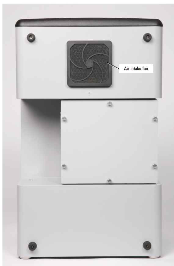
Figure 4-4. Rear panel showing air intake fan. Keep the intake unblocked during operation and accessible for routine filter cleaning (see Cleaning the Fan Filter on page 26).
